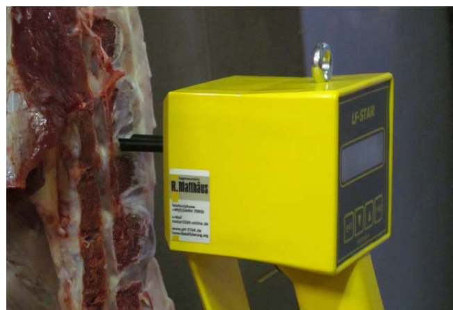
Picture 2: Pistol for measurement of the electrical conductivity of the meat. (Photo: F. Weißmann, TI)
